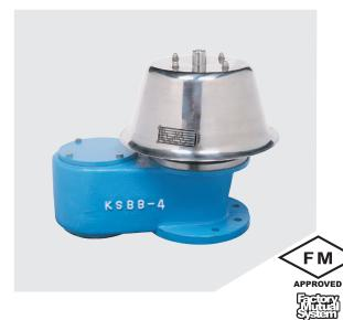
The model KSBB and KSBS pressure vacuum valves are an advanced design for vent to atmosphere applications. Designed manufactured and tested according to the API 2000 code, these valves utilize the latest technologies to provide protection against positive or vacuum over pressure and prevent air intake, evaporative losses of product and help to contain odorous and potentially explosive vapours.
