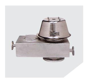
The model KSBBJ and KSJS pressure vacuum valves are an advanced design for vent to atmosphere applications. Designed manufactured and tested according to the API 2000 code, these valves utilize the latest technologies to provide protection against positive or vacuum over pressure and prevent air intake, evaporative losses of product and help to contain odorous and potentially explosive vapours.
